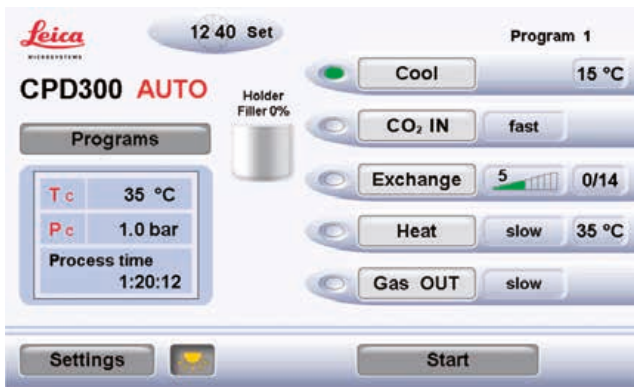
Main display before programming: Left side: Temperature, pressure and process time display, including timer function and holder-filler settings. Right side: Indicates current process status.
